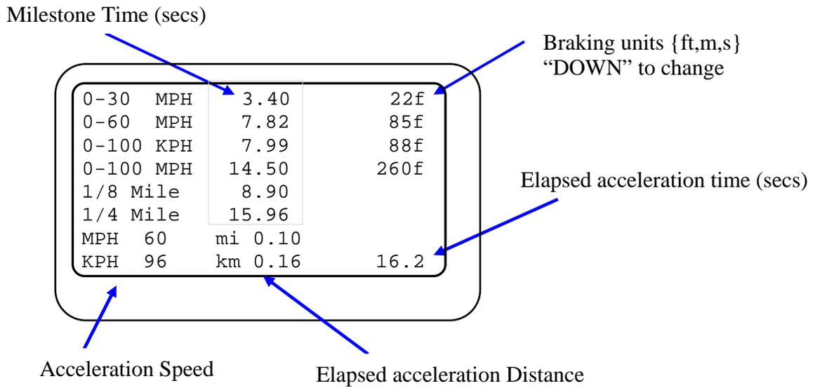
The performance screen is only intended to measure sharp acceleration and braking. It is not meant for any other purpose beyond this. As a result do not leave this screen up while driving as the times and distances will quickly grow too large to fit in the area provided. In general, the elapsed time should not be allowed to exceed 99 seconds. No harm to the gauge will occur; the display will just become overrun with data.
