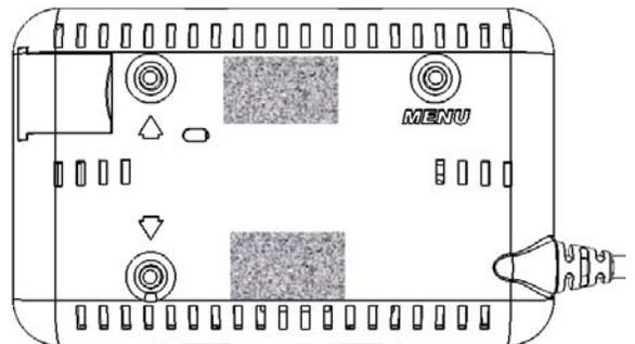
Insure that the surface to which UltraGauge shall be attached is flat, smooth, clean and dry. Once the Velcro has been firmly attached to the back face of UltraGauge, remove the remaining protective wax paper from the Velcro. Press UltraGauge firmly against the desired mounting surface. UltraGauge is now mounted and can be removed and attached repeatedly to configure as necessary.
