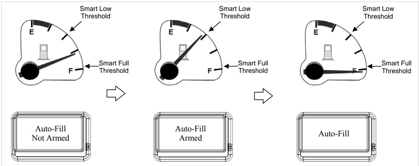
By default the Low Threshold is set to 50% and the full threshold is set to 98%. Setting the Low Threshold too high may cause a false Auto-Fill event to trigger as a result of gas sloshing around in the fuel tank.
