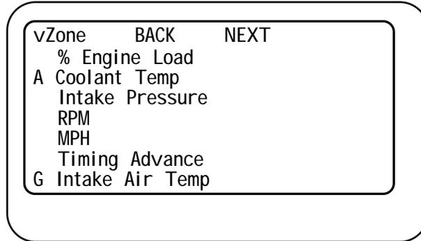
Once a gauge has been assigned to a zone, it is saved. The UltraGauge configuration is stored in non-volatile memory so that it is preserved through car start/stop cycles or the unit is unplugged. The configuration remains until the user chooses to change it.
