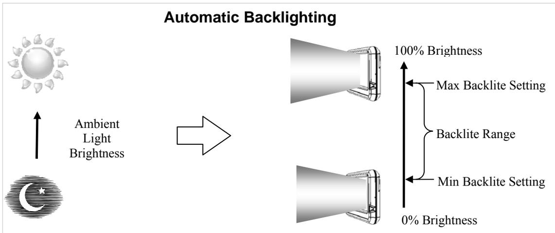
The sensitivity to the Ambient light can be adjusted via the **Ambient Sensitivity** menu setting. This setting allows UltraGauge to better adjust the Backlight brightness depending on the Vehicle's ambient light. For example, vehicles with tinted windows or with smaller windows will have overall lower light levels and an increase in sensitivity would be recommended. See the **Ambient Sensitivity** setting for more detail.
